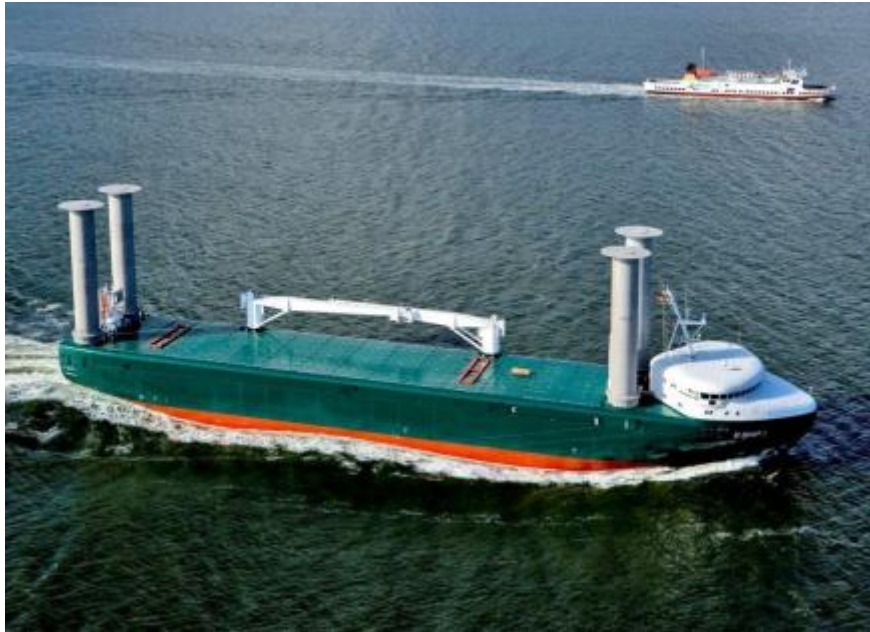
Figure 3: Rotor-ship E-Ship 1 in sea trials (Source: Cassenswerft, 2011)
